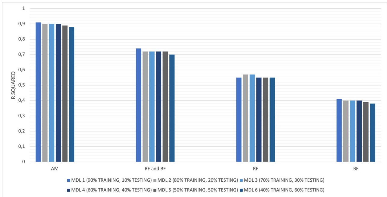
Figure 26: Histogram of R^2 obtained for hip joint. Best results are achieved if one considers all the six muscles with R-Squared around 0.90. R-Squared obtained from the two muscles that cross the hip joint together reaches values close to 0.70, while if RF and BF are considered alone for the regression, the R-Squared obtained is lower than 0.60.
