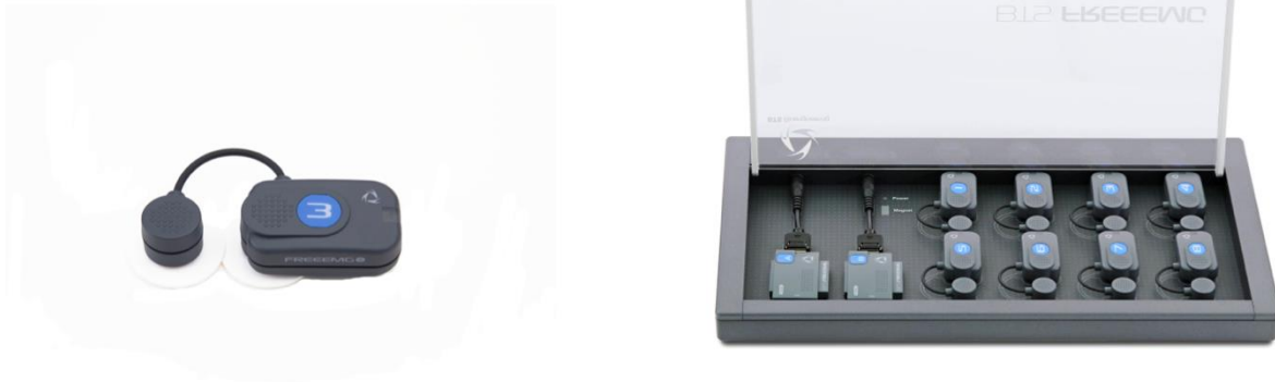
Figure 7: BTS Bioengineering FREEEMG surface electrodes. At left: one of the six surface electrodes used. It is of easy placement and being wires free they let a more comfortable walking task. At right: it is showed the charging box BTS electrodes.
