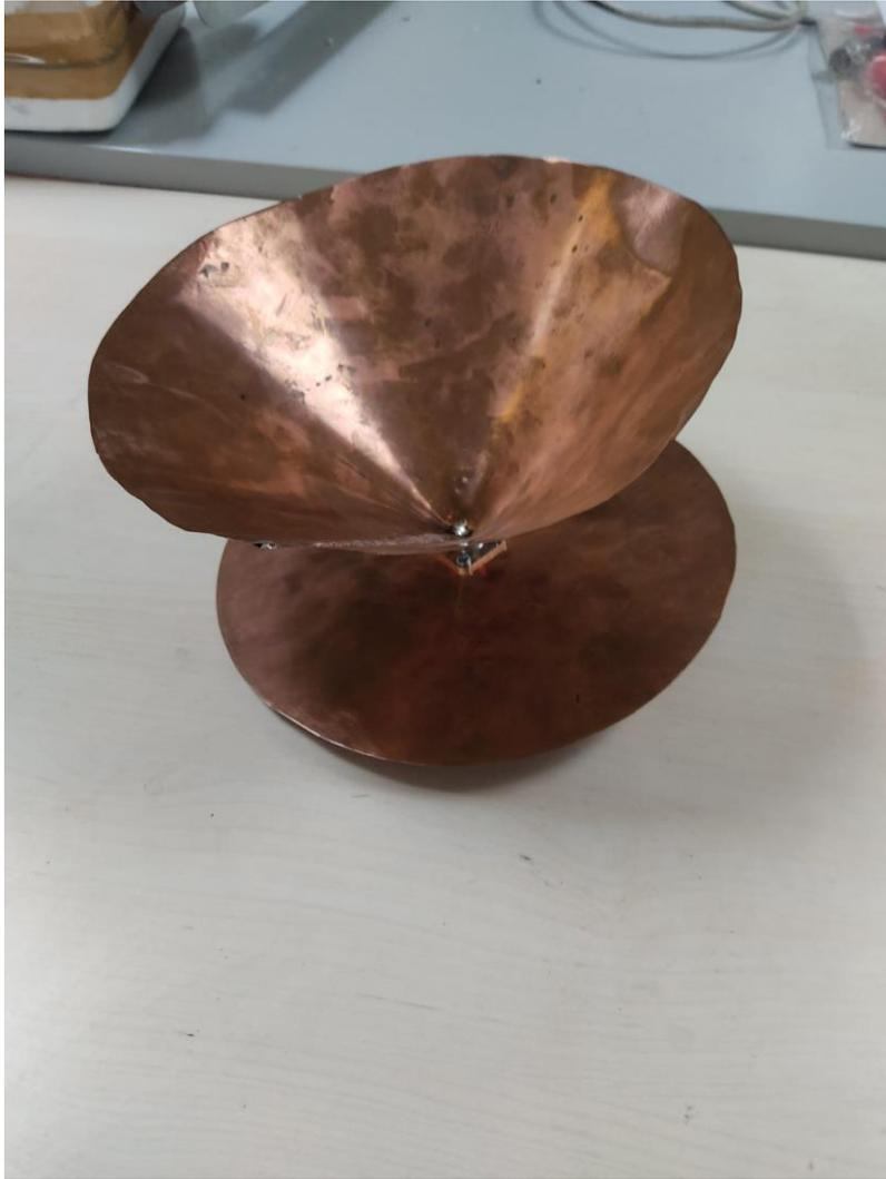
Figura 2.4 Antenna conica
