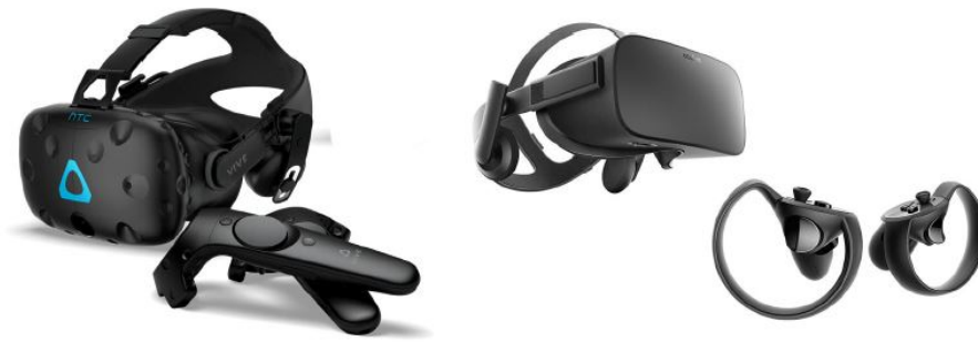
Figure 2.4: Example of full immersive VR headsets, HTC Vive (left) and Oculus Rift (right). Figure adapted from [71], [72].
