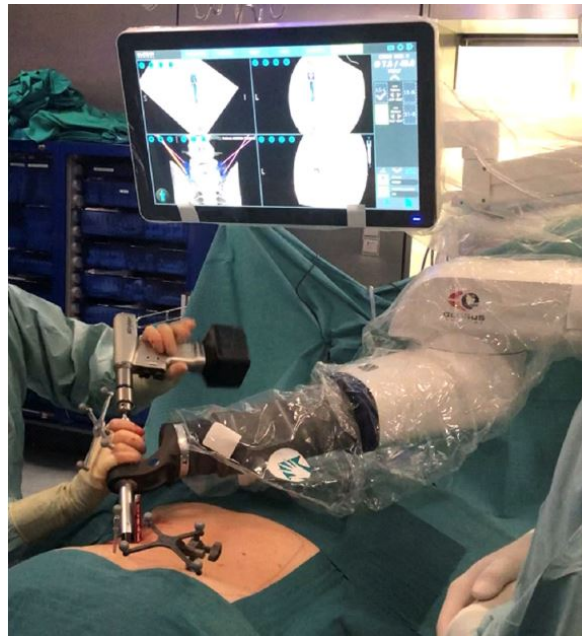
Figure 1.2: The Excelsius GPS (Globus Medical, Inc., Audubon, PA, USA) surgical system allows to guide pedicle screw insertion using a patient-mounted reference array. Figure adapted from [21].
