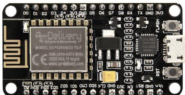
FIGURA 16 MICROCONTROLLORE ESP8266 [65]
