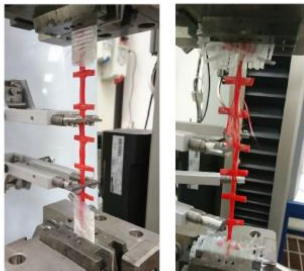
Fig. 3. Tensile test setup and typical failure mode of glass yarn.
