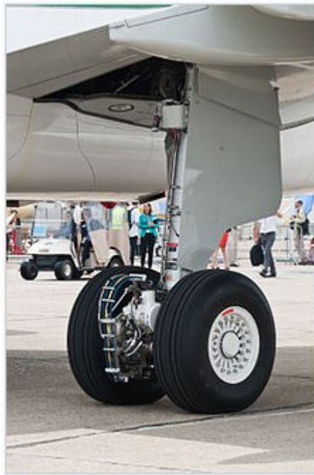
Figure 12: EGTS installed on an Airbus A320 (Wikipedia)
