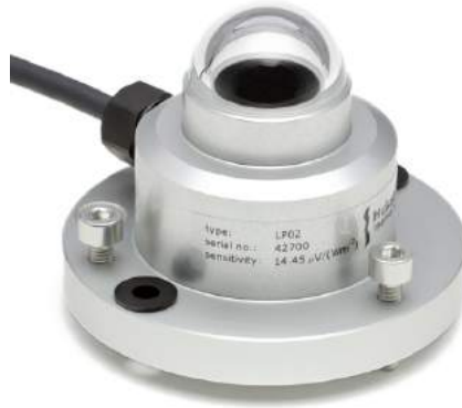
Figura 4.8: Piranometro Campbell Scientific LP02 [89]
