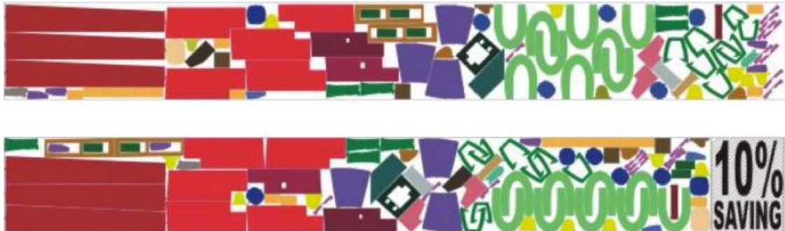
Figura 1.36: Nesting (fonte jetcamcomposite.com).
