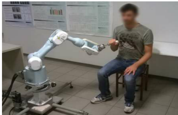
Figure 1.7.: The MitsubishiPA10-7 robot platform.
