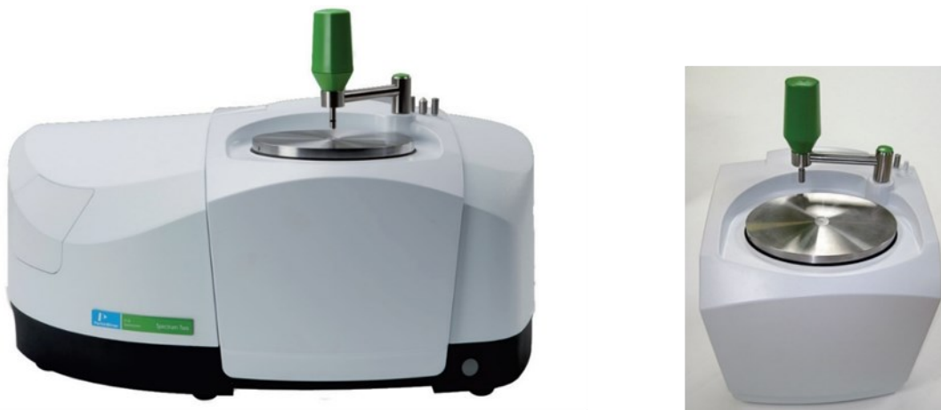
Figure 2.1 Spectrum Two by Perkin Elmer (on the left), Universal Attenuated Total Reflectance (UATR) accessory (on the right) [37].
