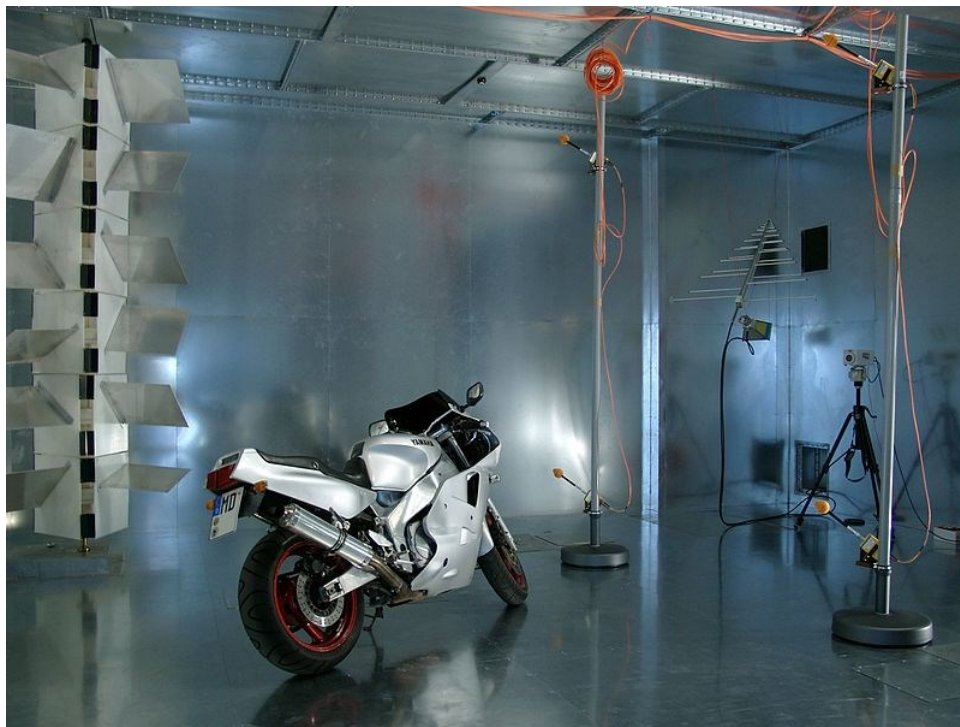
Figure 9 Reverberation chamber at Otto-von-Guericke-University Magdeburg, Germany. On the left side the vertical stirrer mode is placed, ensuring a statistically homogeneous field distribution.
