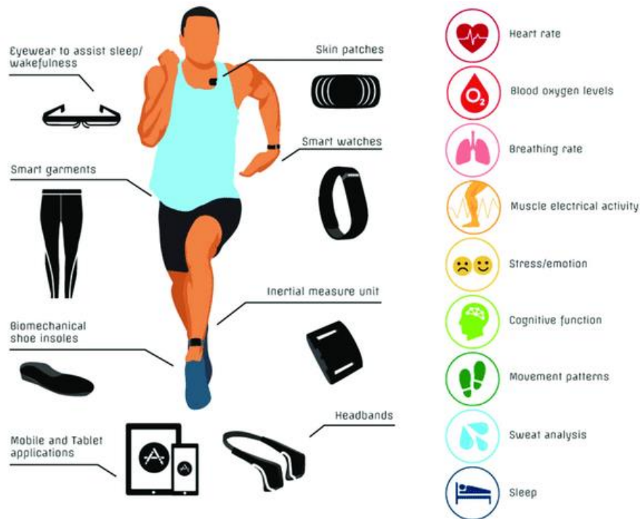
Figure 2: Summary of current technologies for monitoring health/performance and targeted physical measurements [8].
