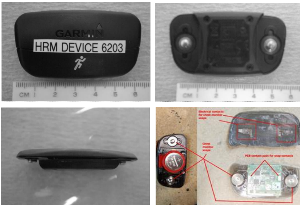
Figure 22: Heart Rate Monitor external and internal photos and dimensions
