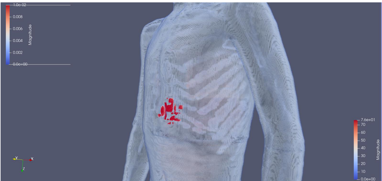
Figure 43: Focus: SAR representation with colour range between [0 - 0.01] and body colour range between [0 – 76] in standard pre-set using “shade” option.
