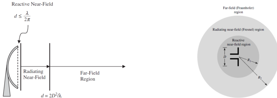
Figure 4: Field regions of an antenna [17].
