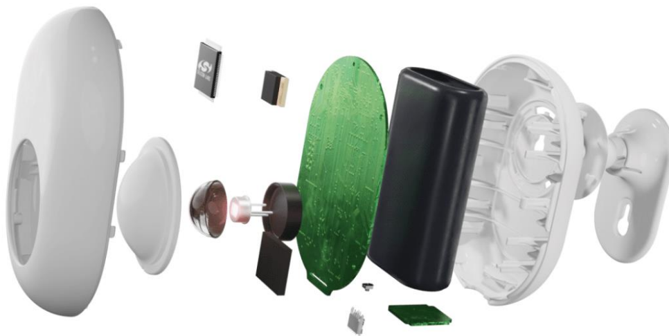
Figura 3.3 – Parte interna Shelly Motion Sensor
