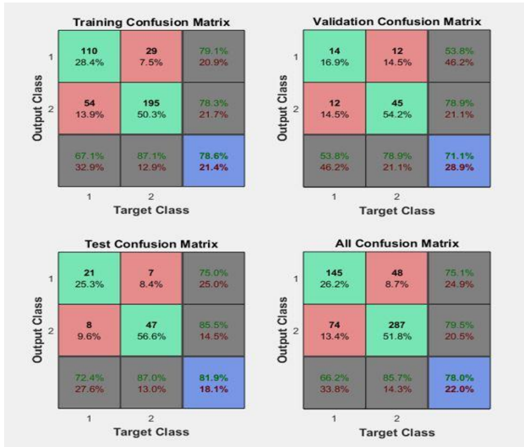
Figure 10. Illustrates the accuracy and precision of the ANN from a confusion matrix. Class 1 = No Stress, Class 2 = Stress. The values in the green boxes represent the true values (upper left, TP and lower right, TN) and the values in the red boxes represent the false values (upper right, FP and lower left FN). The values at the far-right column except the blue box represent the PPV values and those at the lower row represent the TPR values.
