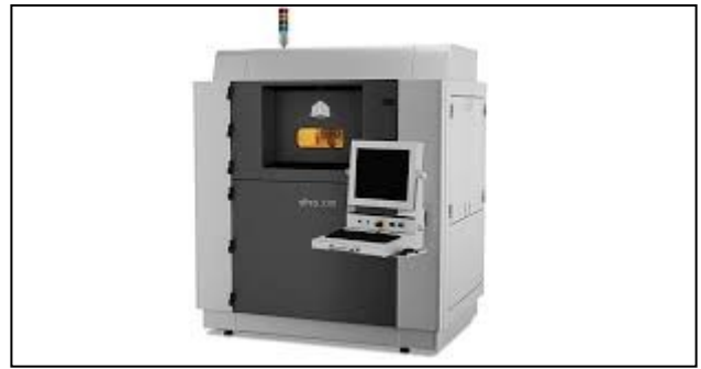
Figura2.6: stampante 3d Systems sPro 230
