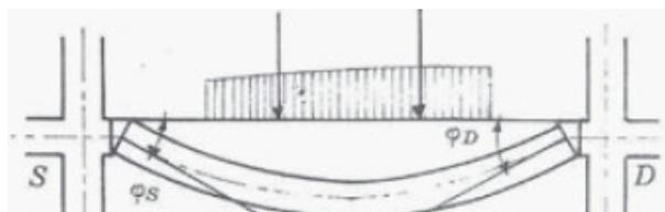
Figura 4.59. Trave uniformemente caricata (PRONTUARIO REP, PROGETTARE CON IL SISTEMA REP: TRAVI REP PILASTRI E SETTI, p. 111).
