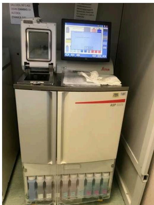
**Figura 10.** ASP6025 Automated Vacuum Tissue Processor
