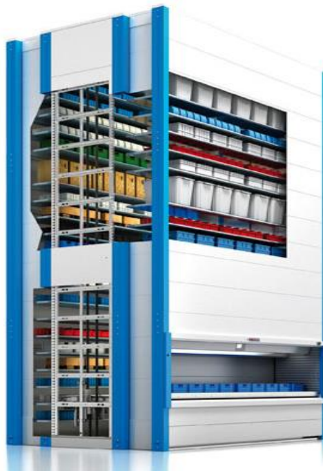
FIGURA 9 VLM (Vertical Lift Module)
