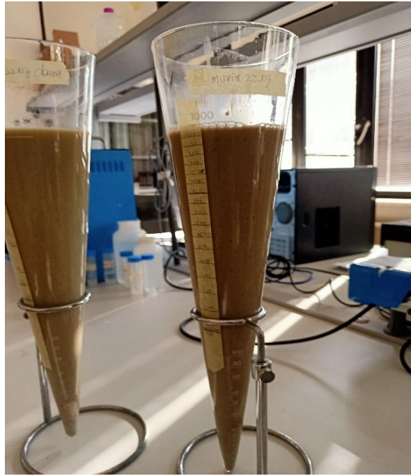
Figure 3-11- Settling test on the liquid part comes from shredding test
