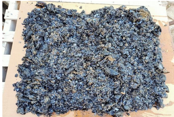
Figure 3-8- crushed shell in the bottom after removal of liquid portion from shredding tank
