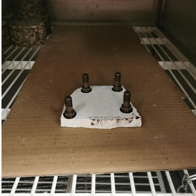
Figura 30: pull stub in camera climatica a 25°
