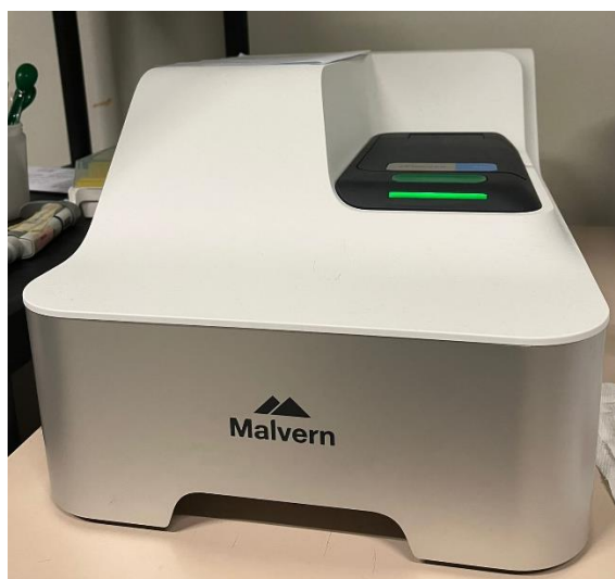
Figura 23. Dynamic Light Scattering Zetasizer pro (Malvern Panalytical)
