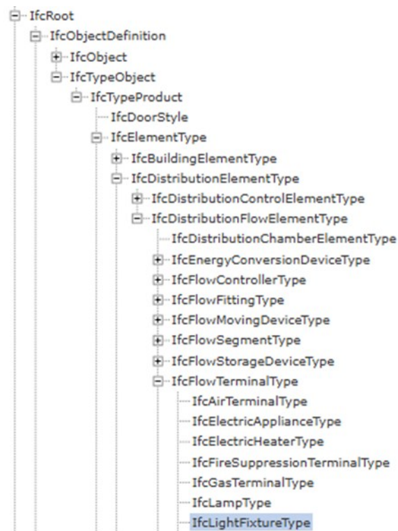
Figura 28b – property set IFC 2x3 per luce di emergenza (sorgente: BuildingSMART International - https://standards.buildingsmart.org/IFC/RELEASE/IFC2x3/FINAL/HTML/ )
