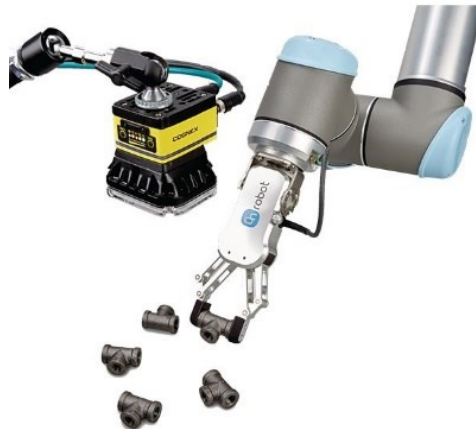
Figure 10. Example of gripper and vision system suitable for UR5.
