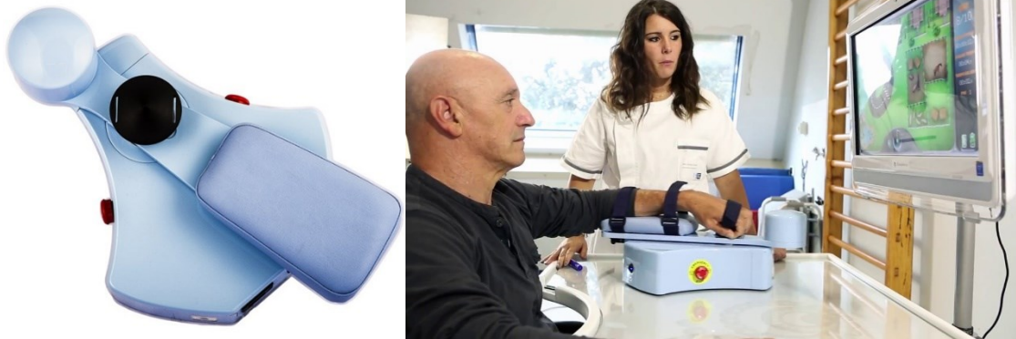
Figure 1. On the left MOTORE used for upper limb rehabilitation. On the right, an application of the medical device during the rehabilitation process.
