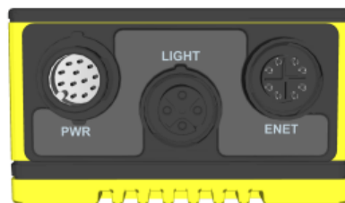
Figure 16. Connectors in Cognex In-Sight 7600.
