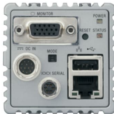
Figure 13. Lighting, digital I/O, serial, Ethernet, and USB buses, as well as display ports for user interfaces.
