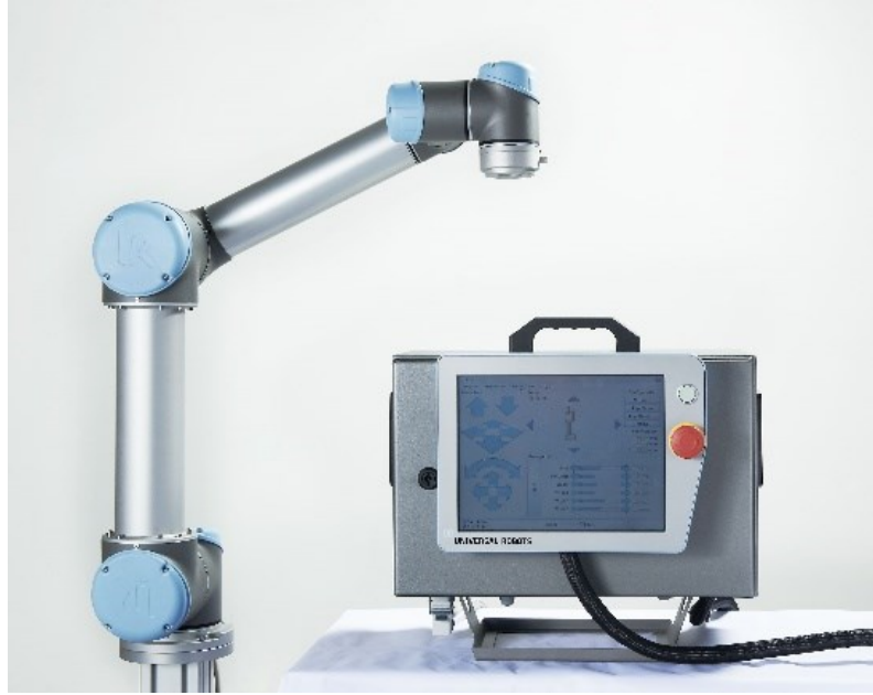
Figure 9. UR10 and teach pendant with Polyscope Robot User Interface.
