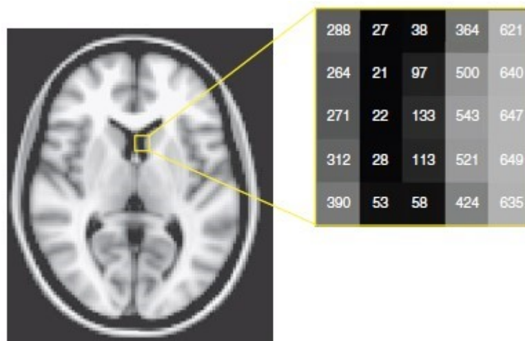
Figure 3.13 The illustration of the image as a graphical representation of a matrix. The grey scale values in the image (left) correspond to numbers for a set of selected voxels (Poldrack et al., 2011).
