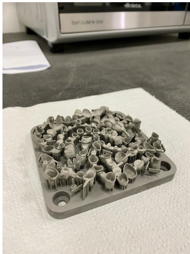
Figure 3.6 CoCr finished SLM prostheses
