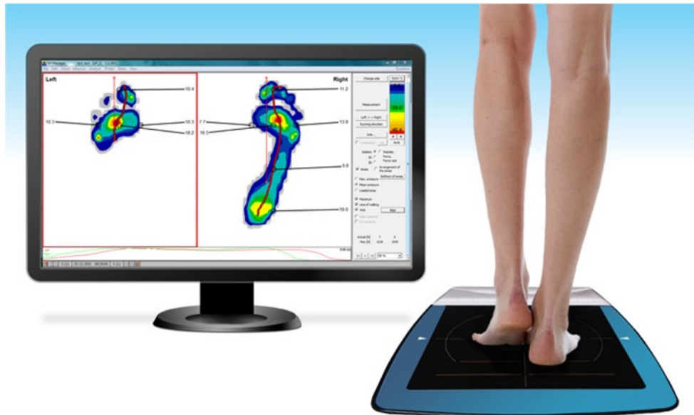
Figure 2.3: Platform-based sensor systems to measure plantar pressure.
