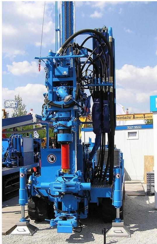
*Fig. 4.1 – Macchina perforatrice per jet-grouting.*
