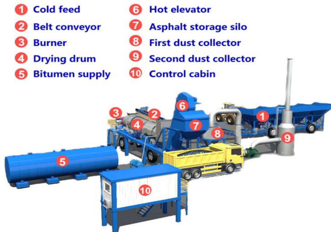
Figure 3. Conventional Drum Mix Plant
