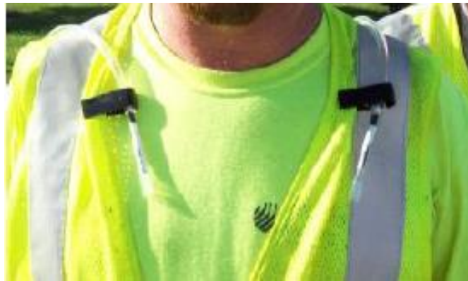
Figure 15. Sorbent tube samplers wore by a worker in Indiana site [25].
