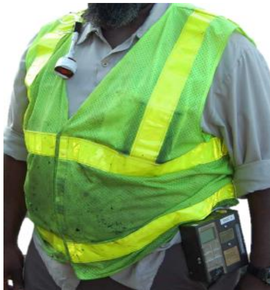
Figure 16. Typical sampler configuration on worker [26].
