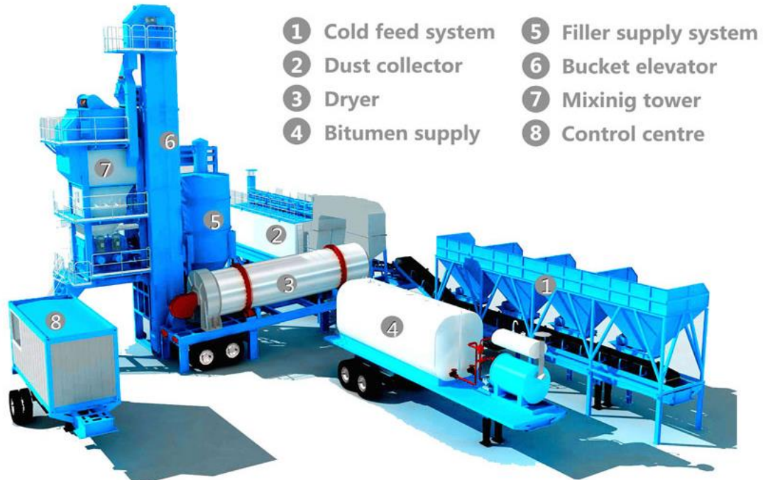
Figure 2. Conventional Batch Mix Plant
