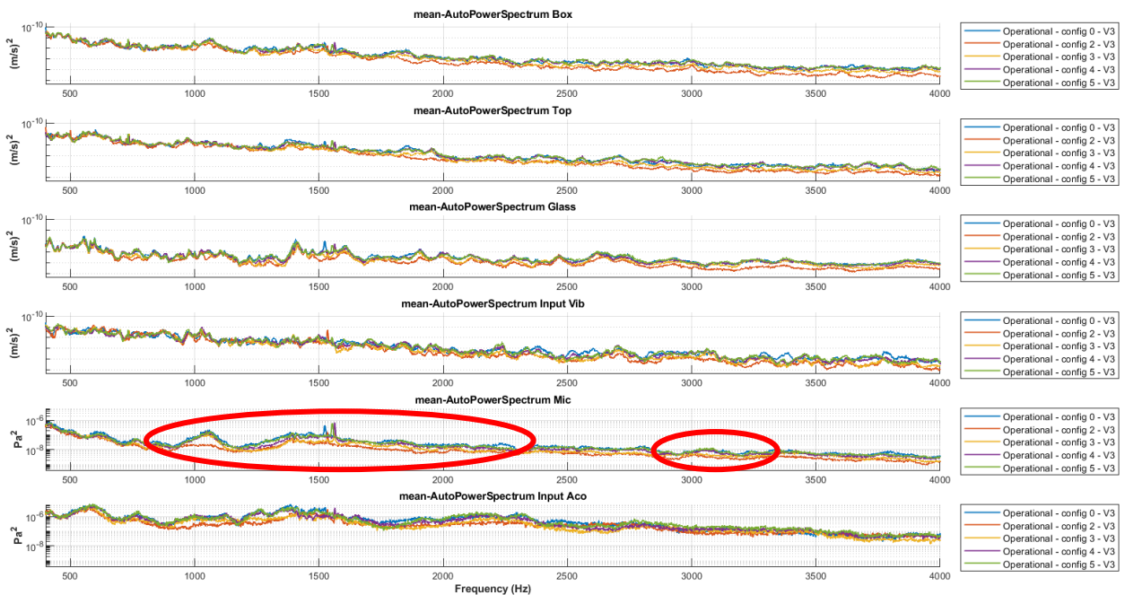
Figura 6.35 Operative Test – Autopower range 400-4000 Hz – config0, config2, config3, config4, config5
