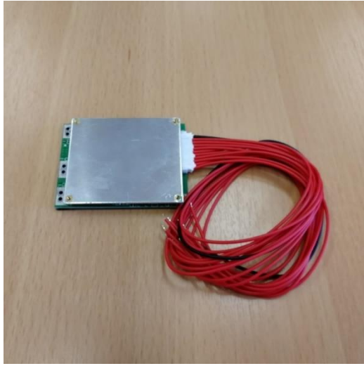
Figura 2.4 – BMS 36 V 35 A 10S
