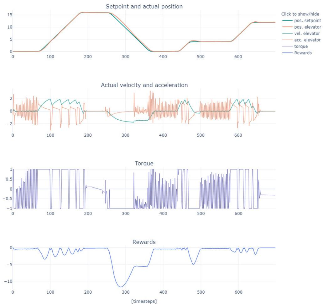
Fig. 37: Trajectory, velocity, acceleration, torque, rewards of one good policy – DDPG agent
