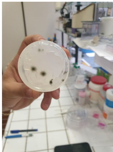
Fig.7: Mold proliferation on hydrogel after 4 days at room temperature
