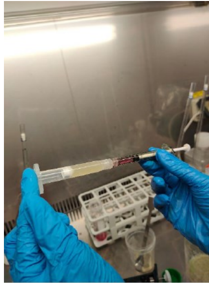
Fig.8: Cellink cartridge loaded whit alginate based bioink and Luer lock syringe with cell suspension.
