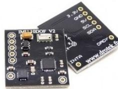
FIGURA 1.10: IMU Drotek 10DoF
