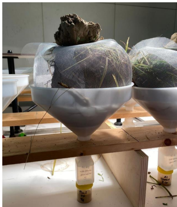
Figure 4. Extraction of the microarthropods using Barlese-tullgren method
