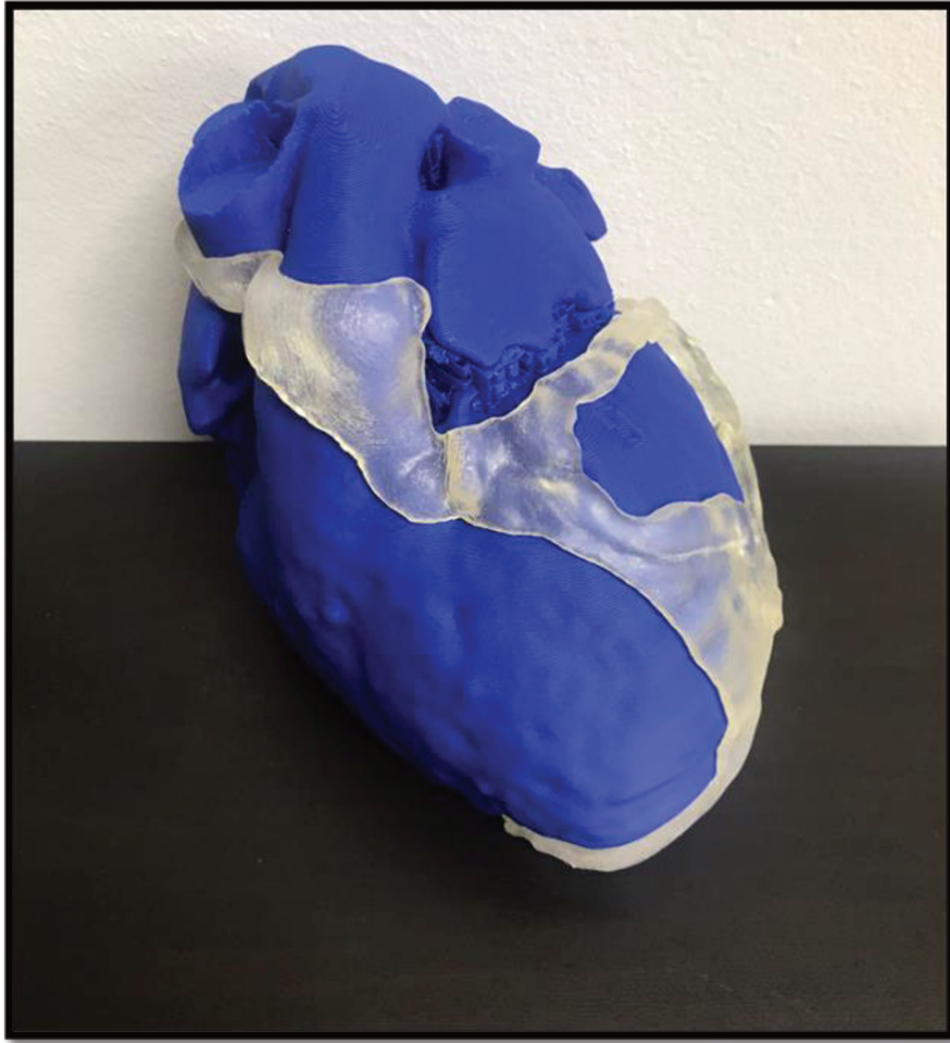
Figure 37. Surgical mask fitting simulation on the heart phantom, previously printed in PLA by PRUSA 3D printer.
