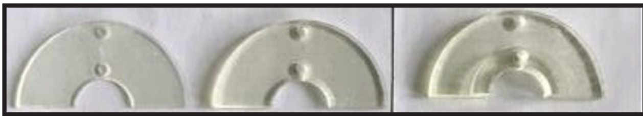
Figure 42. Half circular sector samples of 1 mm, 2.5 mm and 3 mm+ 3 mm of thickness.
