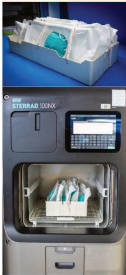
Figure 32. Pouch packaging on the top, Sterrad Vaporized Hydrogen Peroxide Gas Sterilization machine on the bottom.
