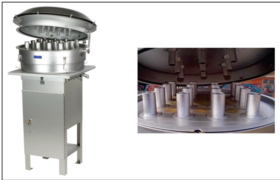
Figure 2.5 - Instrument for measuring the mass concentration of PM_{10} based on the gravimetric principle (left) and detail of the air collection head (right)
