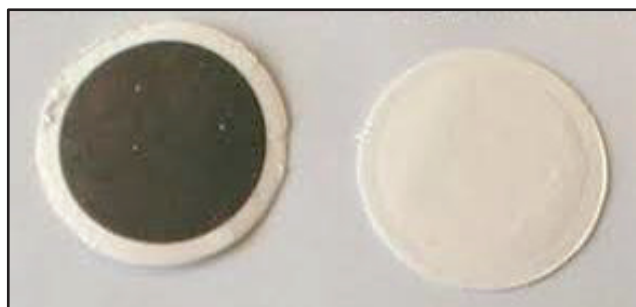
Figure 2.6 - Dirty filter after 24 hours of sampling (left) and clean filter before sampling (right)
