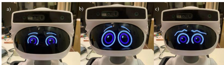
Figure 29. The three expressions that can be visualized on Misty II display according to the predicted TSV value. (a) Joy expression for thermal comfort case; (b) Terror expression for cold discomfort case; (c) Fear expression for hot discomfort case.
