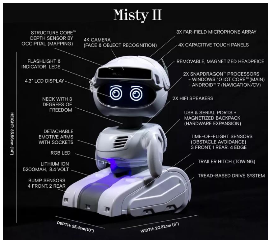
Figure 6. Misty II on-board sensors.
