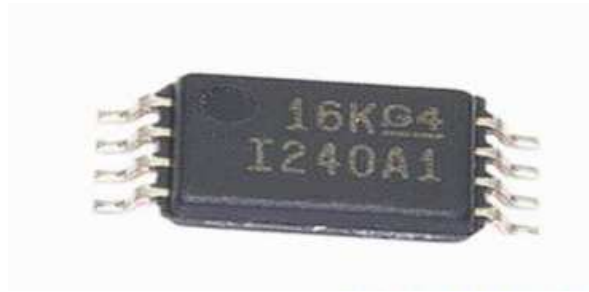
Figure 25: Amplificatore Texas Instruments INA240a1
