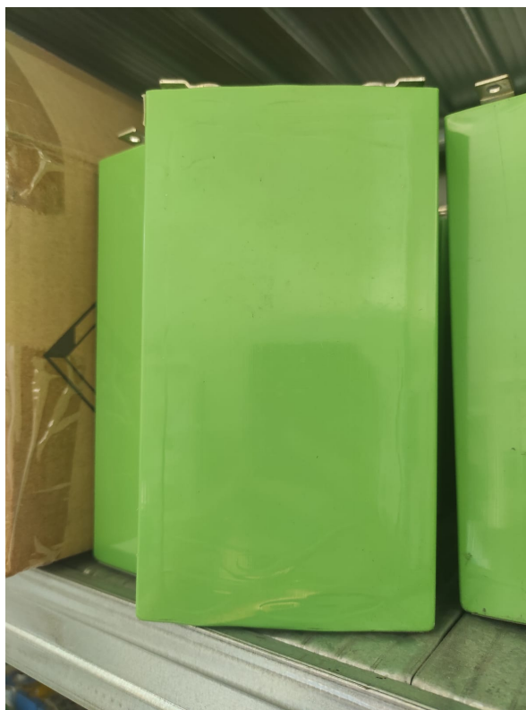
Figure 14: Cella LiFePO4 100 Ah Midac, 49,91mm x 160mm x 116mm
