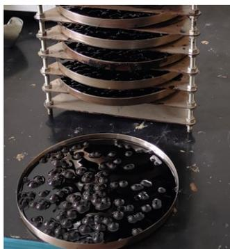
Figura 2.26 bitume post PAV
