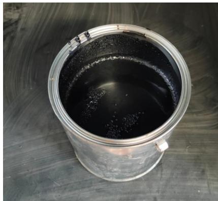
Figura 2.7 bitume SBS-PMB
