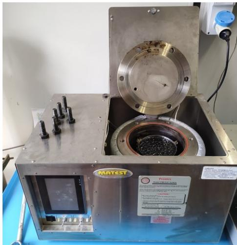
Figura 2.23 Pressure Ageing Vessel (PAV)
