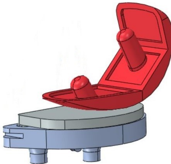
Figure 4.3 Fixed Bearing (Physica ZUK UKA) 3D CAE Abaqus model composed of femoral component (red), fixed-bearing insert (grey), and tibial tray (light blue)
