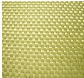
**Figura 10 Fibre aramidiche**
