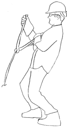
(a) A line worker cutting a large diameter wire with a manual cutter (EPRI, 2001)
