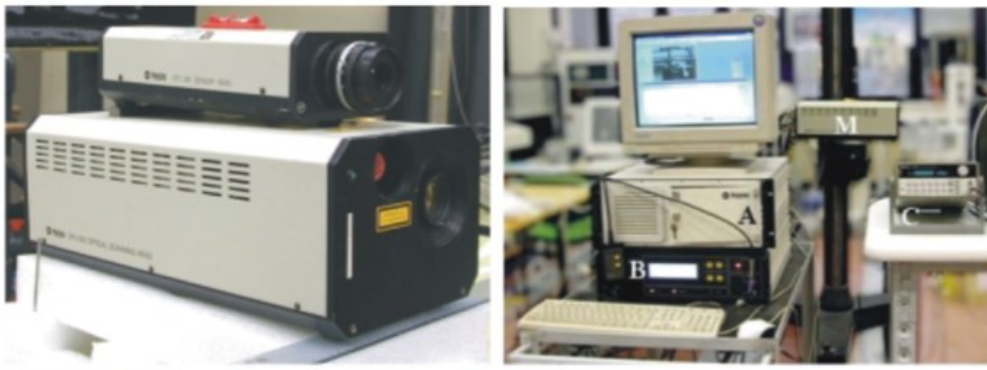
(Figure 5-2) Single and scanning LDV laser heads; SLDV system in the lab. [11.]
