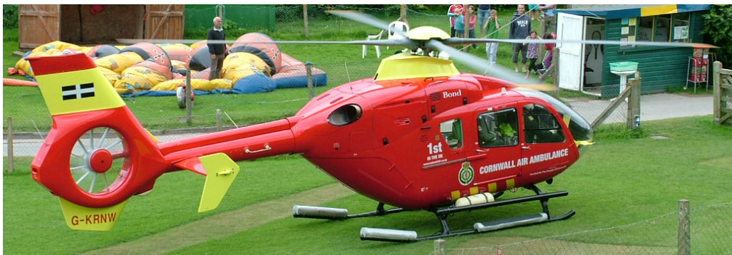
Figure 1.1: Eurocopter EC 135, with a fantail assembly tail rotor (reproduced from https://en.wikipedia.org/wiki/Tail_rotor ).
