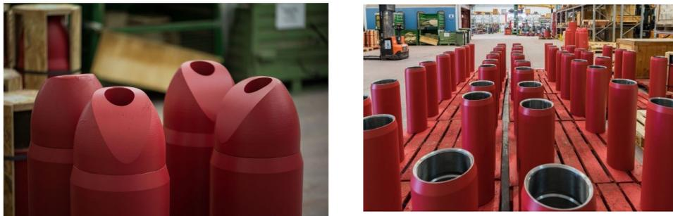
*Figura 14: Casing shoe e Float collar*
