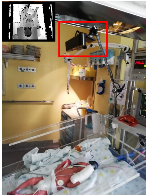
Figure 1.1: Sample of NICU acquisition setup. The Red-Green-Blue-Depth (RGB-D) camera (red box) is at approximately 40 cm over the infant's crib, avoiding hindering the operators [9]. On the top-left corner, an example of acquired depth image is showed.
