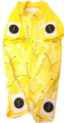
Figure 2.2: Photograph of the smart jumpsuit with four proximally placed movement sensors, by Airaksinen et al. [13].
