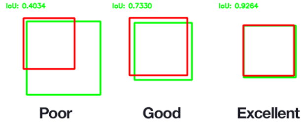
Figure 5.1: Example of computing IoU at different bounding box predictions.
