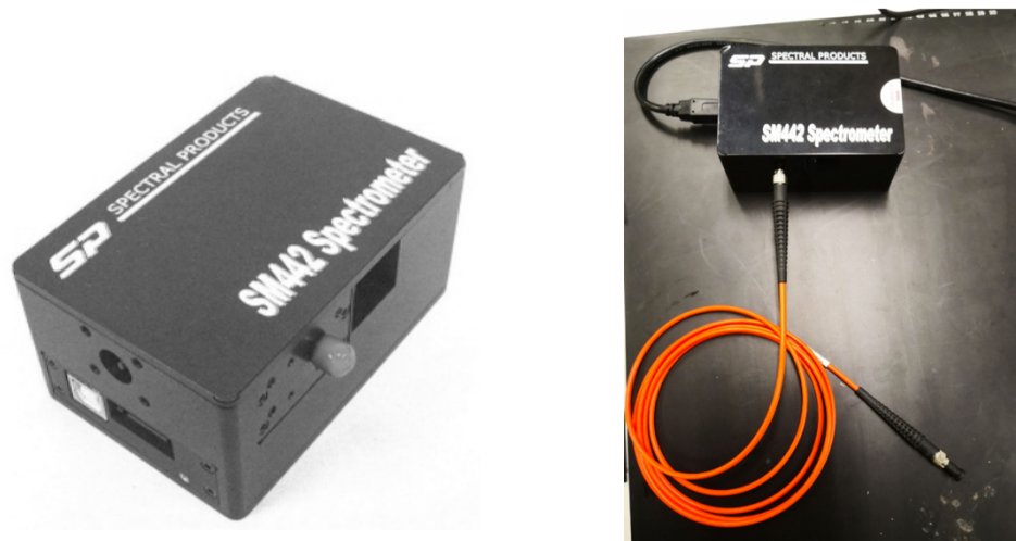
Figure 2.9: SM442 spectrometer, used for spectral characterization of illumination sources in combination with different slit lamp filters
