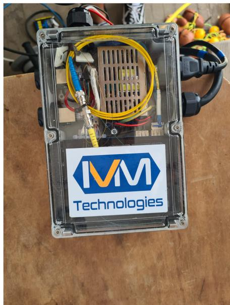
Figure 3.7: Switcher for ROV's communication
