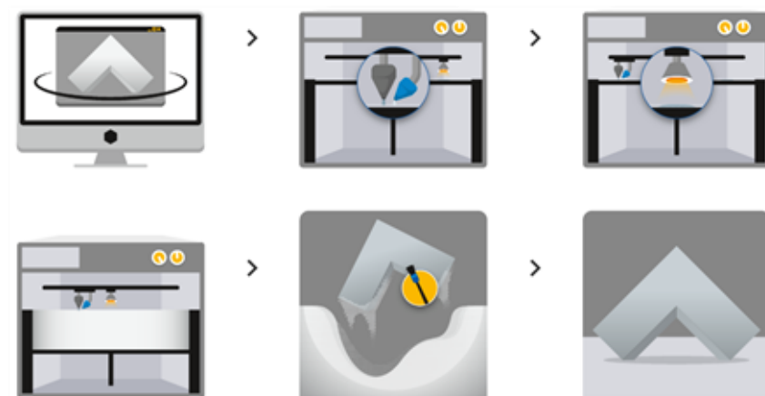
Figure 3. 17 Phases of the Multi Jet Fusion 3D-printing process.
