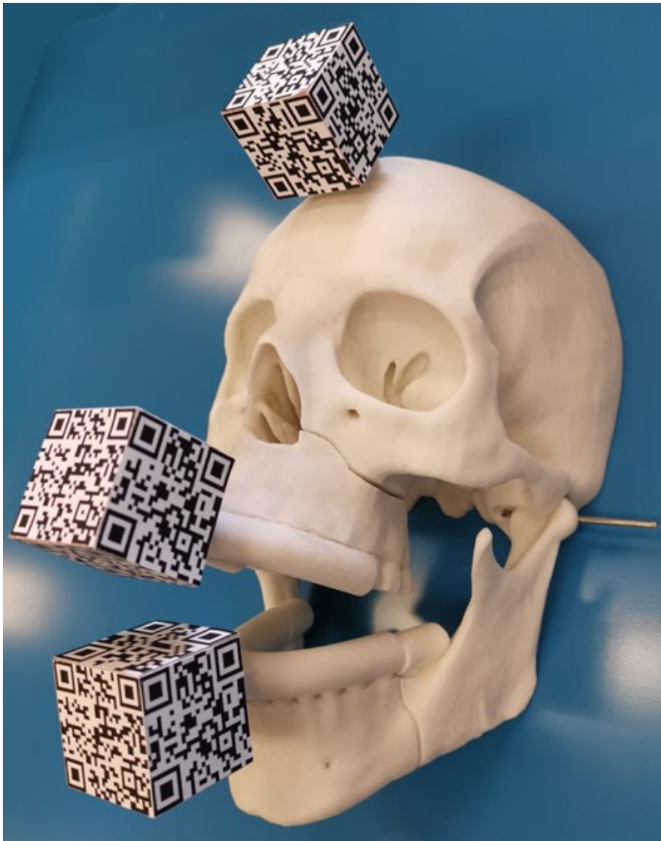
Figure 4. 31 3D-printed phantom with QR codes attached on markers.
