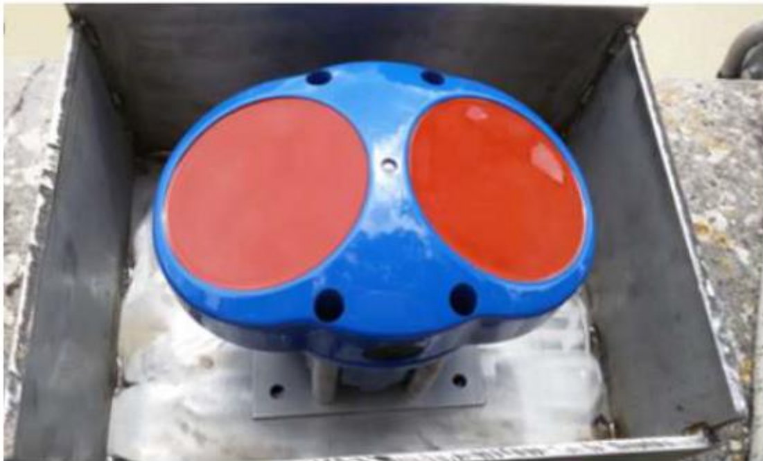
Figure 38. H-ADCP frontal view.
